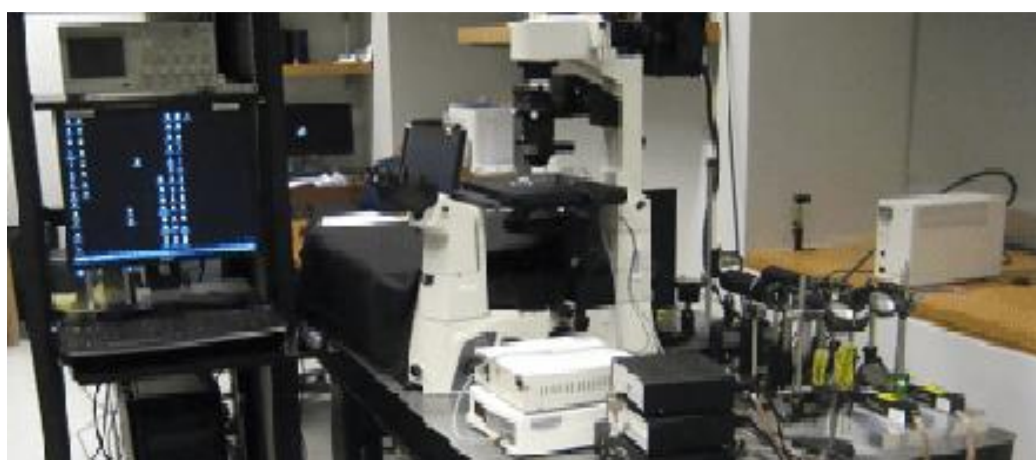
Customized TIRF microscope with the movie-recording software
